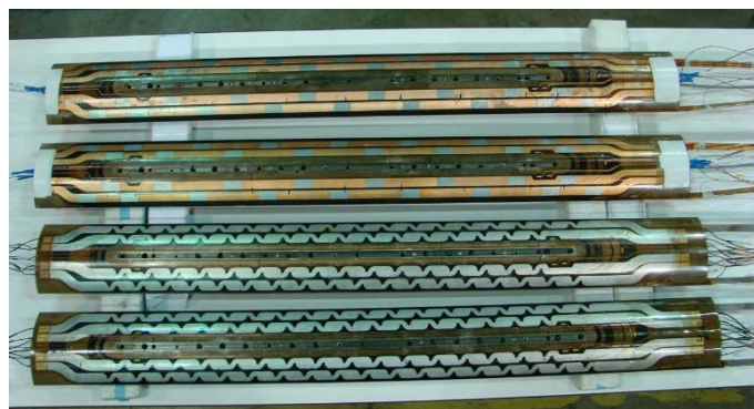
Fig. 6. Coil assembled in the first MQXF short models: from bottom to top, coil 03 and 05 fabricated by LARP) and coil 103 and 104 (fabricated by CERN).
