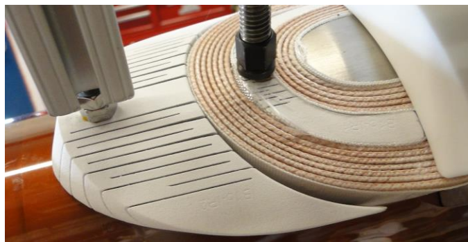
Fig. 1. Picture of ‘accordion style’ end parts first employed in LHQ. The end parts are plasma coated with alumina at 250 μm thickness for additional electrical integrity. The added flexibility accommodates the tendency for cable to separate from the winding mandrel surface also called cable spring-back. The inner end part tightly conforms to cable shape and the outer end part will easily conform to the inner turns after the addition of subsequent tooling and turns.
