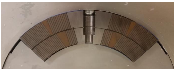
Fig. 2. Picture of MQXFS practice coil 1 within impregnation form block (above coil) and mandrel block (below coil). The beginning of the inner layer to outer layer transition can be seen on the left side of the pole. The coil outer diameter and top keyway groove align each coil during magnet assembly of 4 coils. The coil innermost and outermost radii are 74.75 mm and 113.376 mm.
