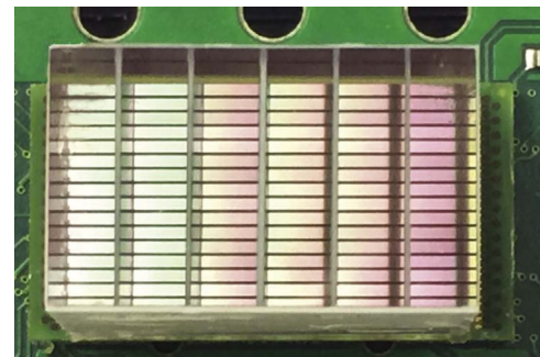
Fig. 2. Photograph of six LFS slabs glued onto a 16 strip MPPC array.
