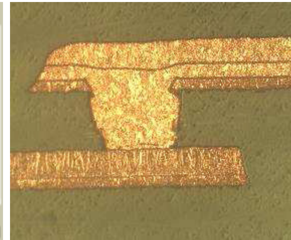
Outer layer impedance too low ( \sim 70\Omega ) due to over-plating
