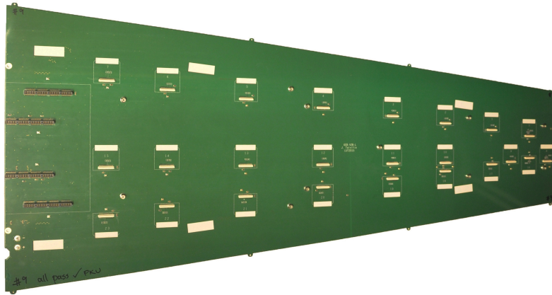
Figure 4. Photograph of the GEB, a 1-m-long multilayer PCB, designed to route the signals of the front-end chips to the OptoHybrid.
