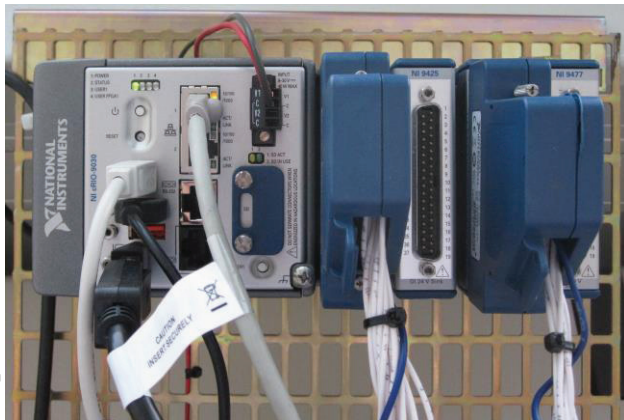
Figure 6: National Instruments cRIO 9030 FPGA controller test bench. The RT-Linux unit is on the left with Ethernet, serial, USB, and video connections. The FPGA unit is on the right with four I/O modules, of which two connected. Each I/O module of this type hosts 32 digital signals.
