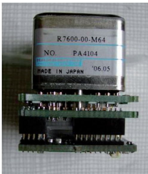
Figure 8. A side view of a MAPMT with a stack of three boards, the PMF, which performs the readout of the fibre signals.
