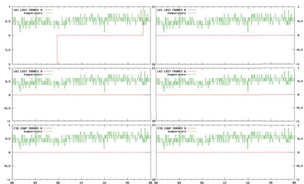
Figure 4: Example of an optical link report, where one of the two optical links has lost a frame (red line in top left plot). The green line shows the card temperature of the day, as a correlation between excessively high card temperatures and transmission errors has been observed.
