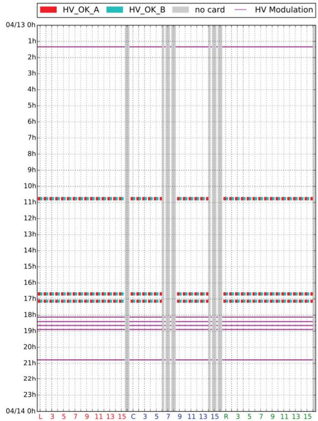
Figure 2: HV Power supply status of three BLM VME crates at Point 1 of the LHC. The x axis is the VME slot number of the acquisition card and the y axis is the time of the day.
