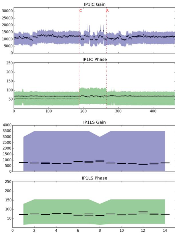
Figure 1: The connectivity test results of all BLMs in Point 1 of the LHC. The measured data points are in black while the shaded regions show the predefined limits for each channel.
