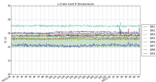
Figure 3: Temperature of one acquisition card in one crate of every Point in the LHC surface buildings.
