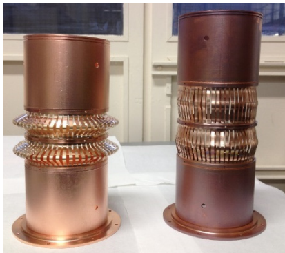
Figure 1: RF deformable bridges for LHC collimator vacuum modules, before and after thermomechanical tests.
