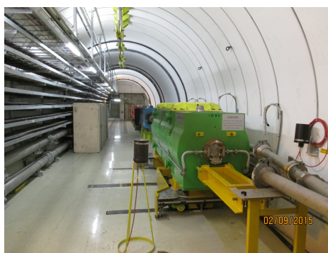
Figure 2: A photo of the TED installed in LHC transfer line TT40. Only the Ti window on the front face of the graphite core as well as the cast iron shielding are visible.
