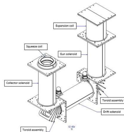
Figure 2: The ELENA cooler magnet system.
