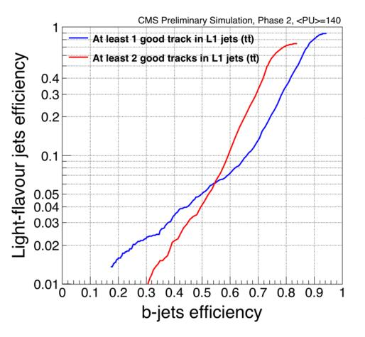
b-jets identification (b-tagging) efficiency versus light-flavour jet (udsg) efficiency are computed using the track counting method based on requiring a minimum value of 3D IP significance.
