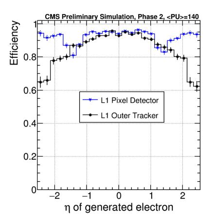
Efficiency of L1 Pixel Electron Trigger as a function of the pseudorapidity ( $\eta$ ) of the generated electron. The efficiency is measured using a single electron sample with  $\langle E_T \rangle$ =35 GeV and  $\langle PU \rangle$ =140.
