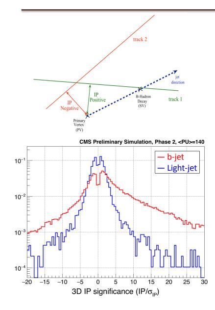
The 3D IP is obtained with the 2D IP in transverse plane and z0 difference between L1 jet and L1PixelTrack as
