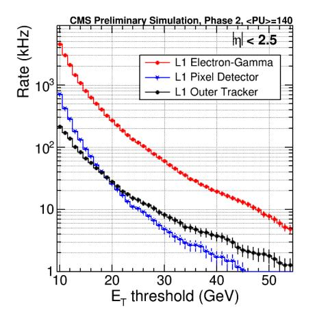
The L1 single  $e/\gamma$  trigger rate as a function of  $E_T$  threshold is shown for  $|\eta| < 2.5$ . The rate is computed with a minimum bias sample with <PU>=140.
