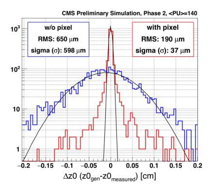
L1 calorimeter jets are matched to L1 tracks from the outer tracker to determine the z position of the jet vertex (\*). For these studies, L1 track-matched jets within 2mm of the L1 primary vertex (\*) are considered. L1 jets are also matched with gen-level information to select only light-flavour jets.
