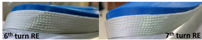
Fig. 9. Cable in contact with the mandrel at the end of two return end turns.
