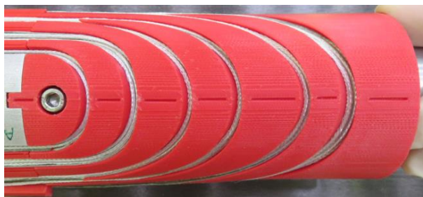
Fig. 10. Final winding of the return end of the design in blocks. The return head is about 130 mm to be compared to the 200 mm of the previous design.
