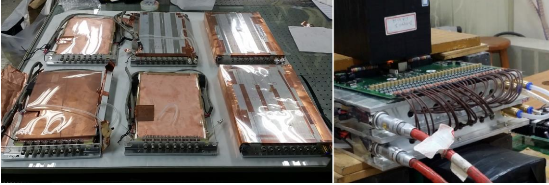
Figure 1. Six RPCs with different gap thickness from 1.0 to 2.0 mm in a step of 0.2 mm.
