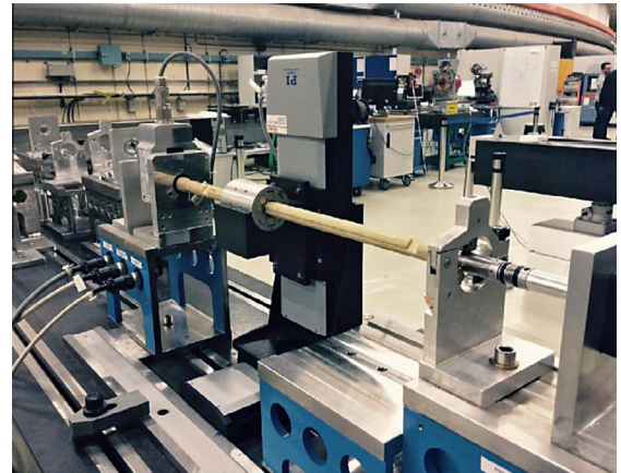
Fig. 5. Test-bench used for calibration experiment.
