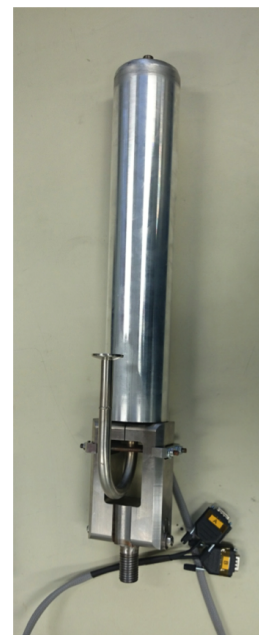
Figure 4: Adjusted insulation break sample including attached tooling for load application and gas dome.
