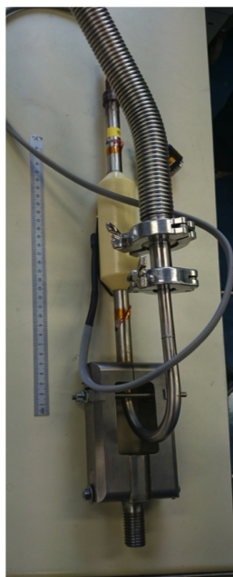
Figure 3: Adjusted insulation break sample including attached tooling for load and vacuum application.
