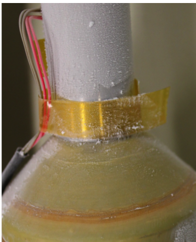
Figure 9: Defective regions observed on the as-tested IB30kV2, by visual inspection.
