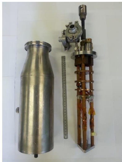
Figure 1. 18kN cryostat. On the left, the female part consisting of a dewar; on the right the male part consisting of inner columns, thermal screens, sample holder and pulling rod.
