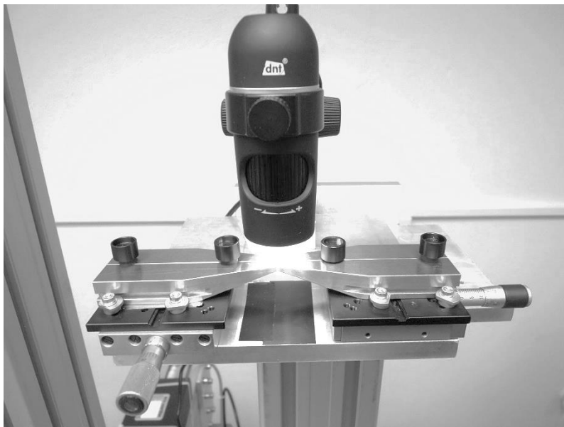
Figure 13: Gluing station consisting of two translation tables (in x-y configuration) and a USB microscope. The fibres are held by soft magnets in the V-grooves of the two mounting plates.
