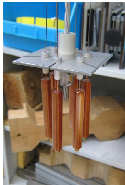
Figure 4: Centring plate and weights for the anodes
