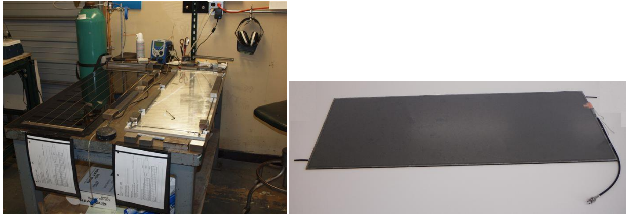
Figure 7. Left: one of the three assembly stations for the construction of RPCs. Right: a completed chamber.
