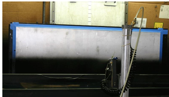
Figure 5. Photograph showing the spraying of a sheet of glass with resistive paint.
