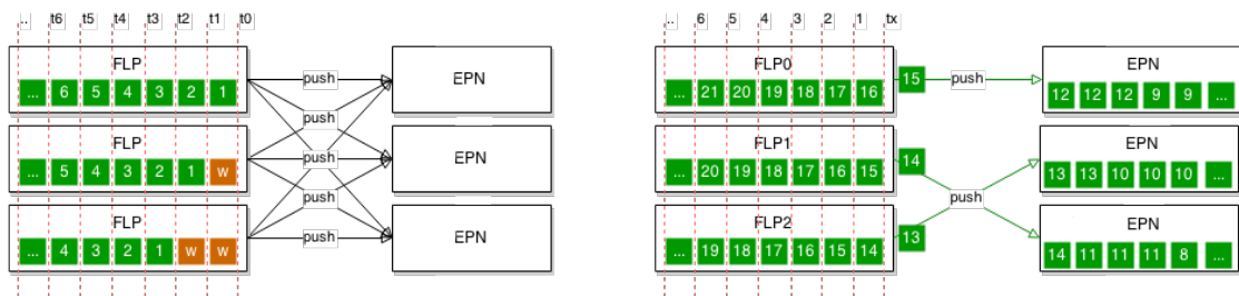
Figure 3. Example scenario of staggering transfers with priority values increasing by 1 for each FLP component (no simultaneous transfers). In this scenario, the first FLP component does not have any delay and can constantly send at full rate. Others delay the incoming sub-time frames until the path to the target EPN becomes free (the delay is shown in the left picture with 'w'). The picture on the right shows the sending pattern when the buffers for the staggering are full - each component can send at full speed and avoid collisions because the destination EPN is different for each sender.
