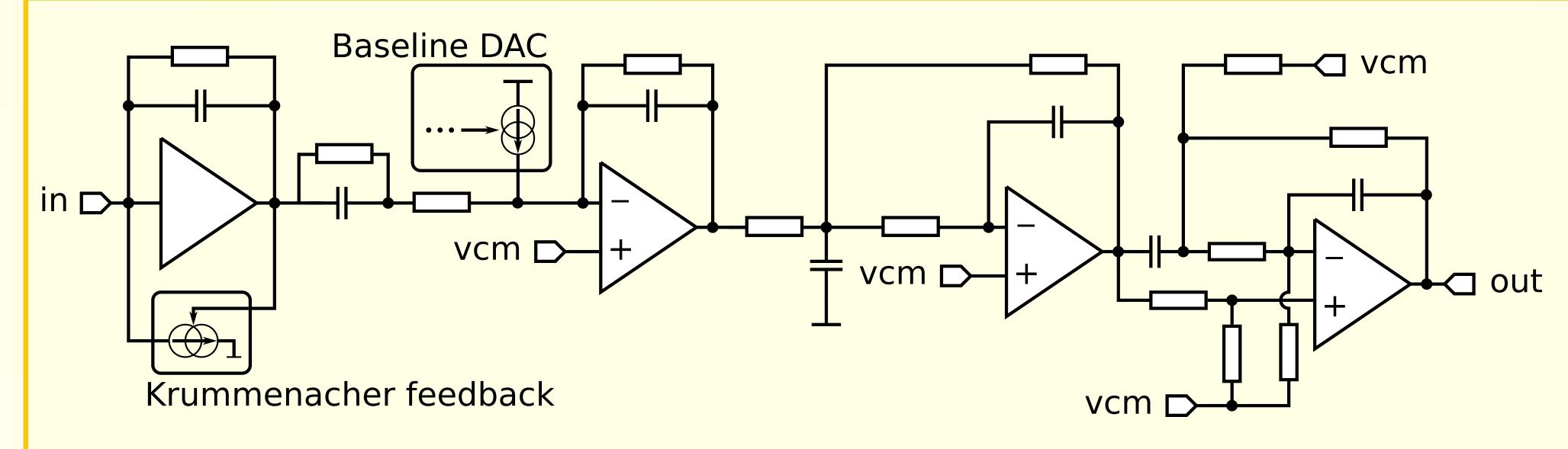
The front-end comprises a charge preamplifier and a fast shaper ( $T_{peak}$ =25ns and fast recovery) required to distinguish pulses from subsequent LHC bunch crossings at 40 MHz. To achieve this, a specific non-standard shaper is required. The prototype front-end (process A) works with sensor capacitances between 5–30 pF.
