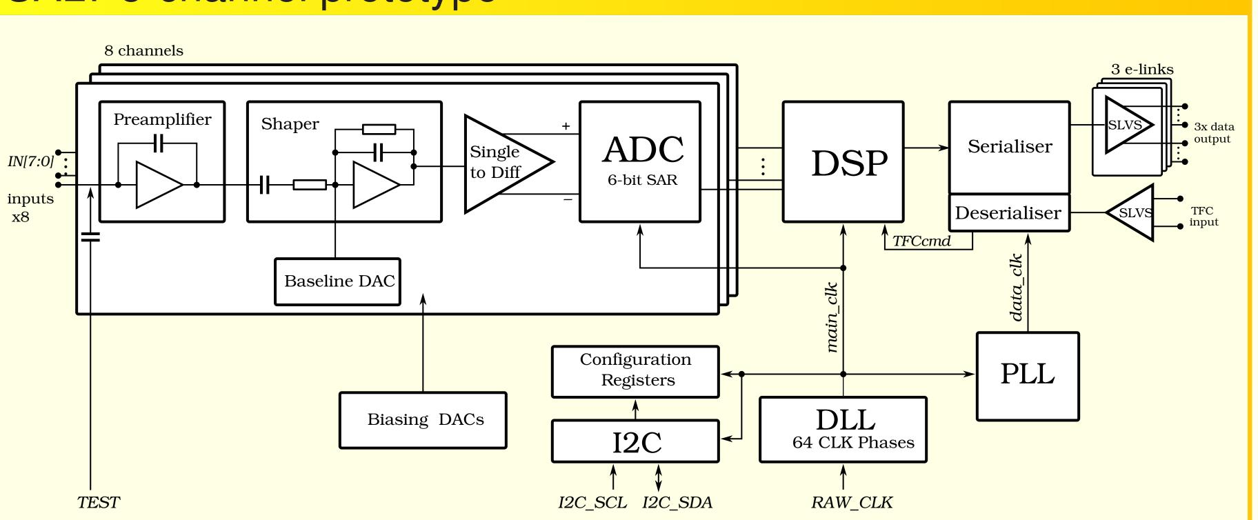
The 8-channel SALT prototype was designed and fabricated in technology B. Basic tests show fully functionality of slow control (I<sup>2</sup>C), input (TFC) and output (data) interface. The PLL based (de)serialisation also works correctly. Other tests are in progress.
