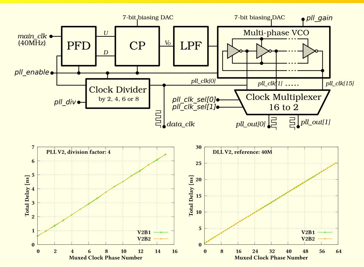
The PLL and DLL were manufactured and successfully measured in both technologies A & B. See talk by Mirosław Firlej: Development of a low power Phase-Locked Loop (PLL) and Delay-Locked Loop (DLL) in 130nm CMOS technology.
