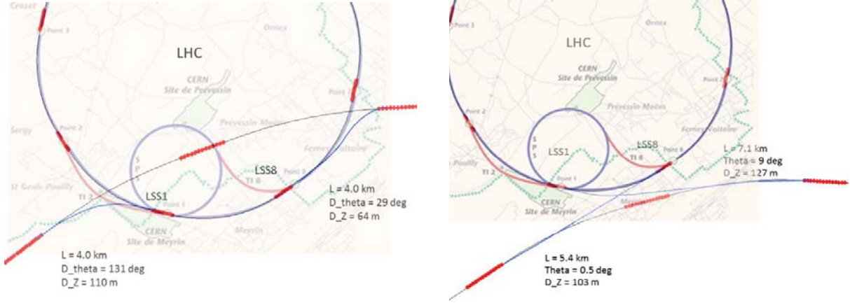
FIG. 8: Possible configurations of FCC-hh with LHC used as “High Energy Booster” (HEB) injector [23].
