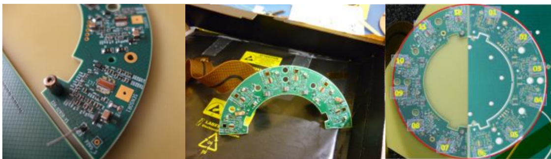
Figure 2. Pictures of the front-end electronics. On the left side: the front-end circuit is glued to the PCB, the square metalised place for the diamond sensor is visible; On the center: the front-end PCB with 6 ASICs mounted, the flex part of the PCB connecting the main part with the part designed for an optical transmission is visible; On the right side: two front-end PCBs with numbering of the sensors, the boards are mounted on two parallel planes positioned around the beam pipe.
