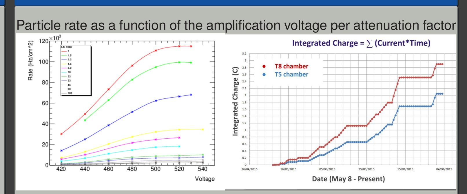
**Particle Rate for T-chambers and Integrated Charge**
