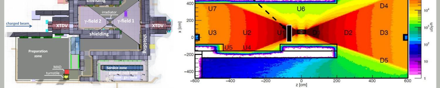
The high source activity produces a **very intense background gamma field** allowing to accumulate doses equivalent to High Luminosity LHC (HL-HC) experimental conditions in a reasonable time. **Filter system** permits attenuating the photon rate in several steps to reach **attenuation factors** of several orders of magnitude (~10<sup>4</sup> - 10<sup>5</sup>)
