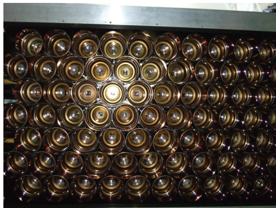
Fig. 1. Pixel Hybrid Photon Detectors (HPDs) integrated in one box of the RICH 1 detector. The hexagonally packing is clearly visible.
