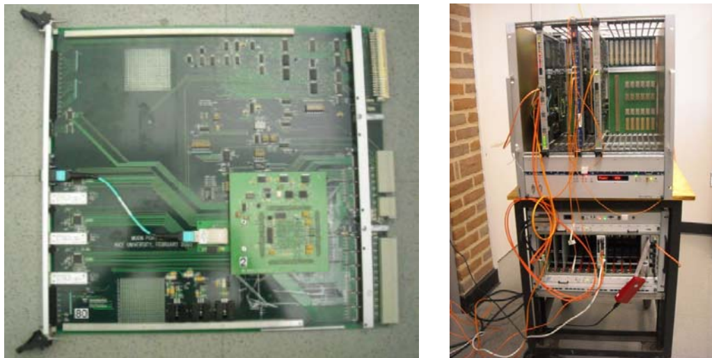
Figure 4: Upgraded MPC baseboard (left) and a test stand at Rice University (right)
