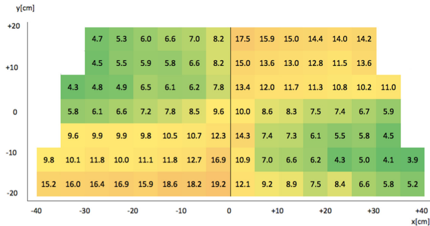
Fig. 10. Mapping of the resistivity on one readout layer. The impedance is measured between the HV supply point, on the top-left side or bottom-right side for the two sectors, and the indicated spot on the layer, resulting in a systematic asymmetry.
