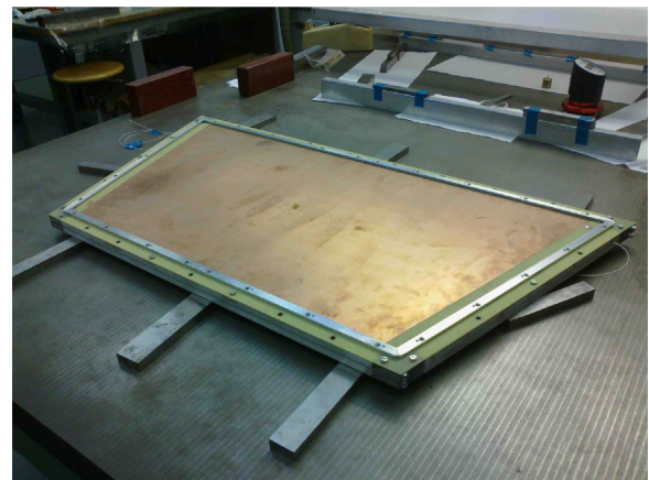
Fig. 15. Mesh frame glued to the drift panel, in the centre of the drift electrode the small insert (see text) is also visible.
