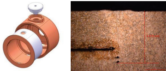
Figure 4: Stage 1: assembly of the water circuit inside the drift tube body.
