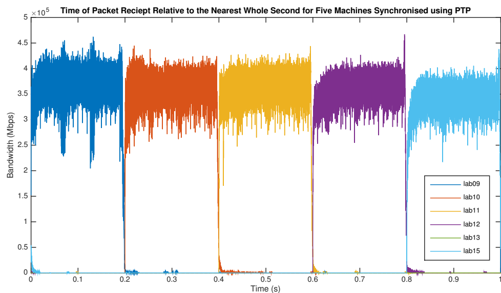
Figure 3: Number of packets received at each time relative to the previous whole second for machines synchronised using PTP
