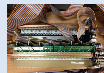
After assembly, 600 connections on each motherboard and end board were again **quality controlled** for continuity.
