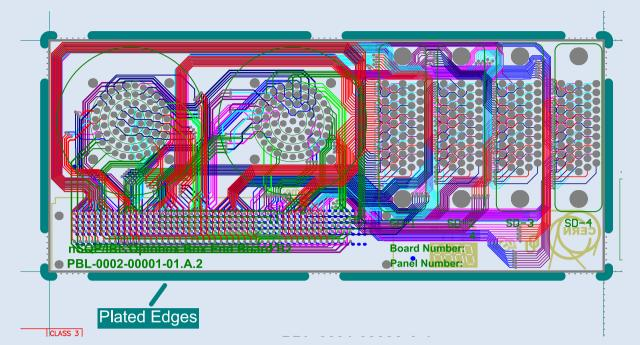
Printed circuit board (PCB) fabrication panel for the end board. Solid copper internal layers and edges provide electromagnetic **shielding** and **grounding**. ENIG (gold) plating provides high **reliability**. The boards passed **quality control** before assembly.
