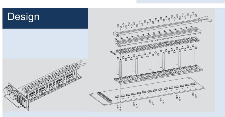
**Mechanical** drawings show the **custom design**; a slot and spring mechanism keeps the opto-boards in place and allows for easy loading and extraction.
