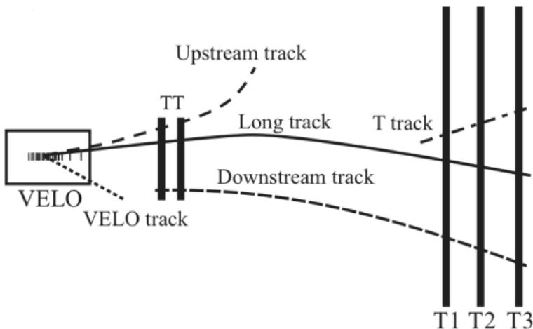
$K_S^0$  candidates are separated according to where in the detector they decay, within the VELO (Long) or downstream from the VELO (Downstream), due to different detection efficiencies and detector resolutions.
