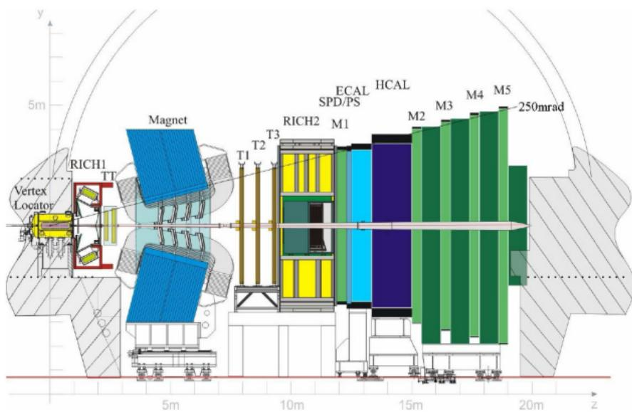
Single-arm forward spectrometer with acceptance  $2 < \eta < 5$ , designed for high precision measurements of decays involving b and c quarks<sup>[1]</sup>.
