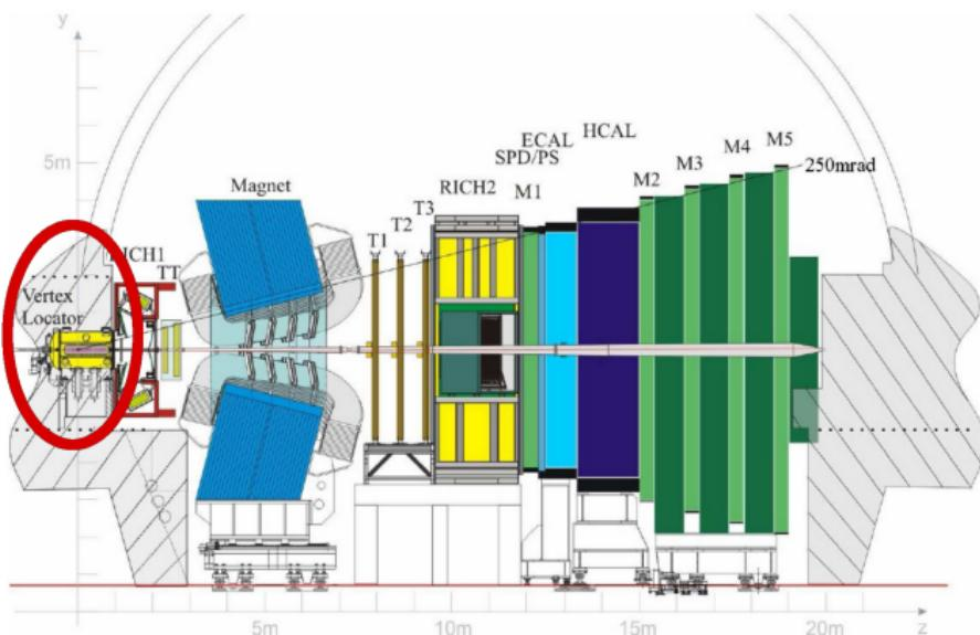
Provides fine tracking about the interaction point, achieving impact parameter resolutions of  $\sim 20 \text{ } \mu\text{m}$  for tracks with  $p_T > 1 \text{ GeV}$ <sup>[2]</sup>.
