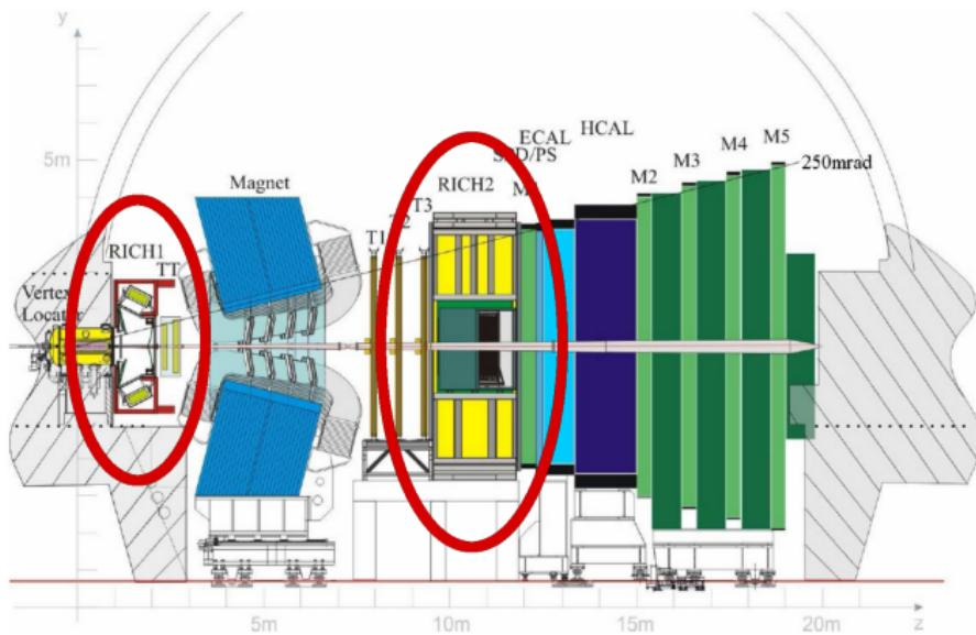
Two RICH detectors provide particle identification, with excellent separation of  $\pi$  and K over a wide momentum range<sup>[3]</sup>.
