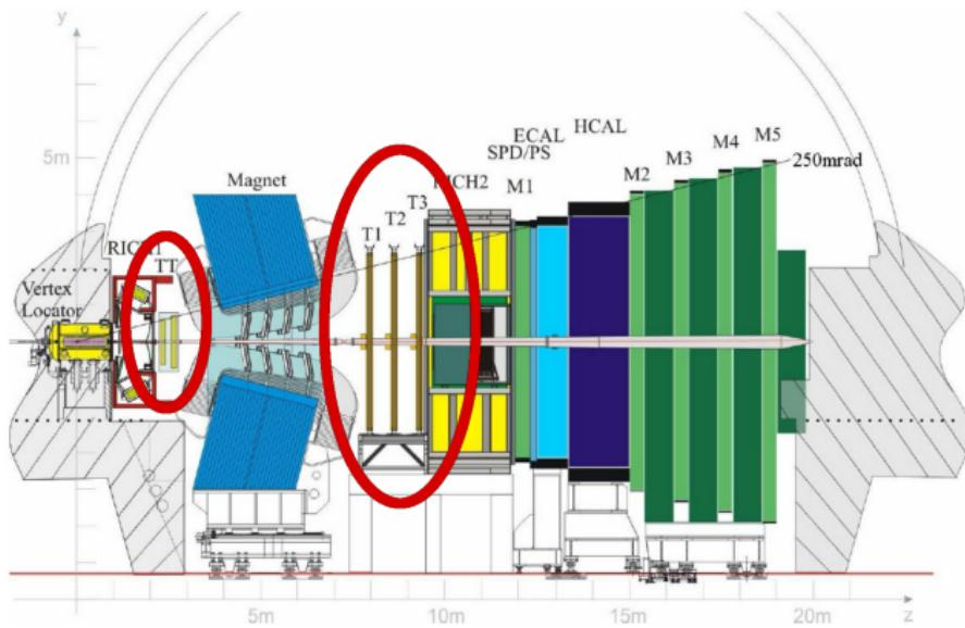
Tracking stations before & after the dipole magnet achieve momentum resolution of  $\sim 0.5\text{-}0.8\%$  [4].
