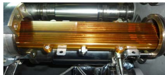
Figure 3. Electrical insulation system
