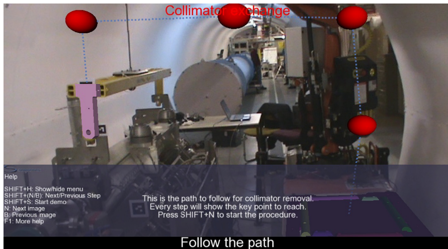
Fig. 7. Instructions showing the path to follow for the collimator removal. This step is displayed after the hook–spreader alignment and before the actual collimator removal. When the operator press the right key, the first key point starts to flash, showing the order to follow.
