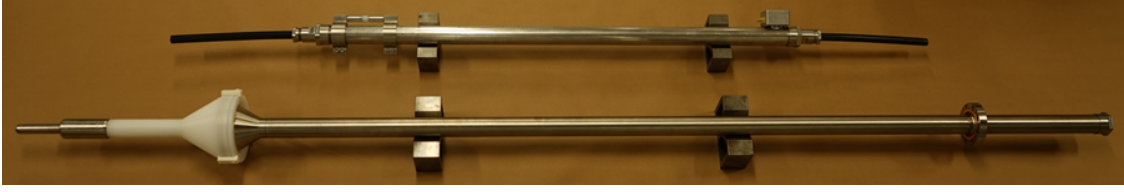
Figure 9. The feedthrough for the LBNE 35 ton prototype.
