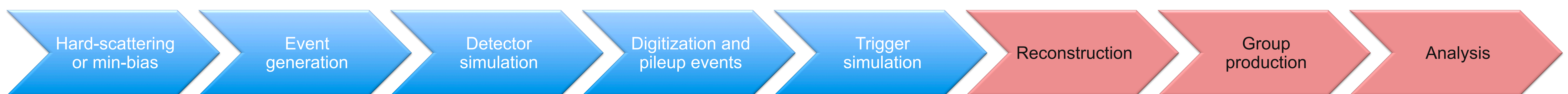
Figure 1: The Monte Carlo workflow is composed of many steps: generate or configure hard-processes, hadronize signal and minimum-bias (pileup) events, simulate energy deposition in the ATLAS detector, digitize electronics response, simulate triggers, reconstruct data, convert the reconstructed data into ntuples for physics analysis, etc. Outputs are merged and/or filtered as necessary. The real data are processed through the same workflow chain starting from the Reconstruction step.
