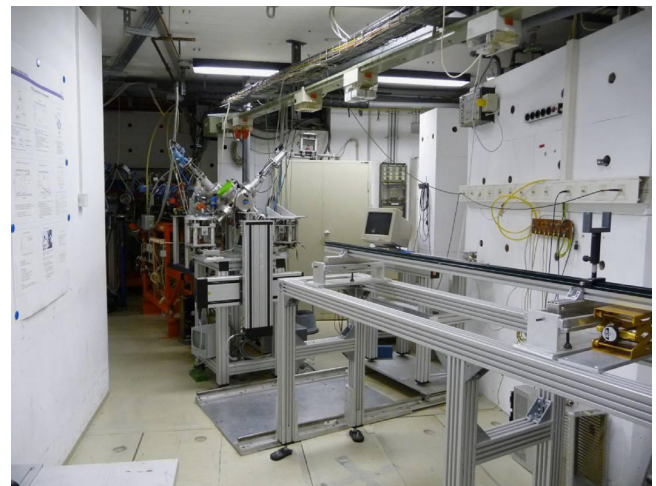
Fig. 2. Picture of the optical bench. The instruments are placed on a shifting trolley (off-axis in the picture) equipped with mechanical locks to ease the positioning reproducibility.
