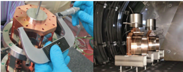
Figure 3: Dimensional checking during bars assembly (left) and compact couplers vacuum brazing (right).
