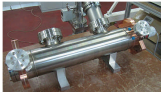
Figure 4: Assembled PETS and leak test.
