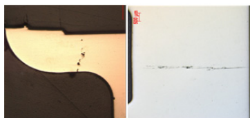
Figure 5: Left, LME in the HAZ. Right, shows a macro-inclusion in the bulk material of the flange.
