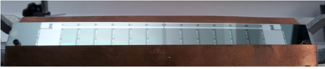
Fig. 10. Photograph of a thermo-mechanical sample. The circuits that mimic the ASICs are clearly visible.
