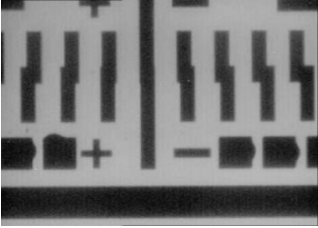
Figure 7: Infra-red image of a well aligned vertical alignment vernier scale. A perfect alignment is reached if only the central long aluminium lines of both wafers completely overlap. For each 6\mu\text{m} of misalignment, the lines that completely overlap are shifted by one to the left or right.
