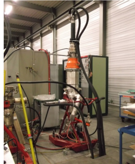
Figure 5: Cryomodule and RF system layout in the LSS4 cavern (left) and a 400 MHz Tetrode amplifier under test (right).
