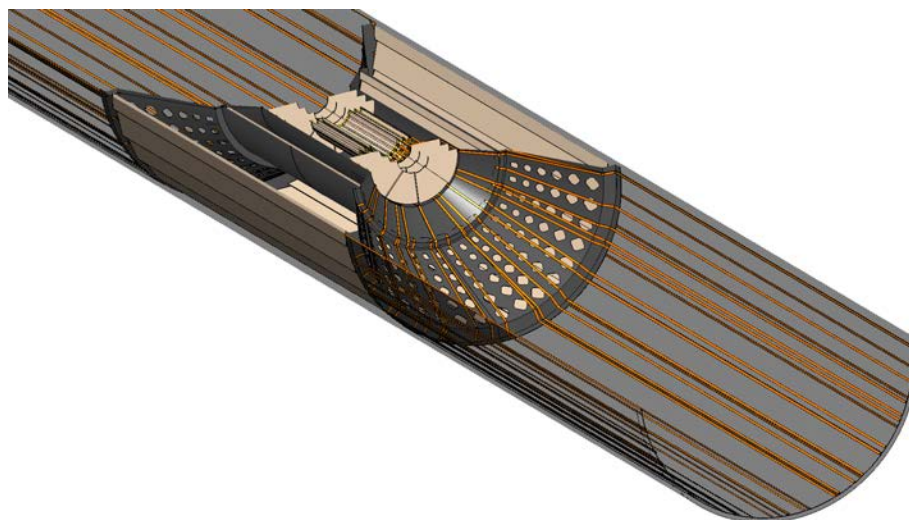
Figure 50: Global vision of all the cables mentioned before in one half of the Inner Support Structure of the inner region. It includes the VXBD, the Vxec, the SIT1 and SIT2 cables.
