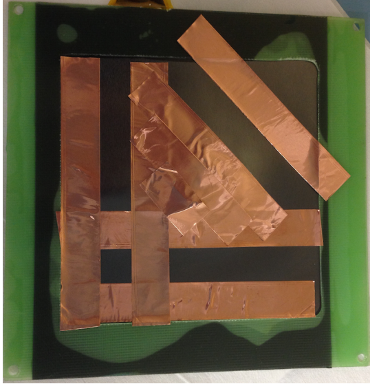
(a) ^{10}\text{B}_4\text{C} coated cathode
