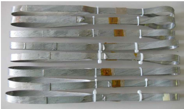
Fig. 4. LHC busbar cable test loops for current decay constant measurements. The cable splices have been prepared with different cable overlap lengths ranging from 3 to 120 mm.
