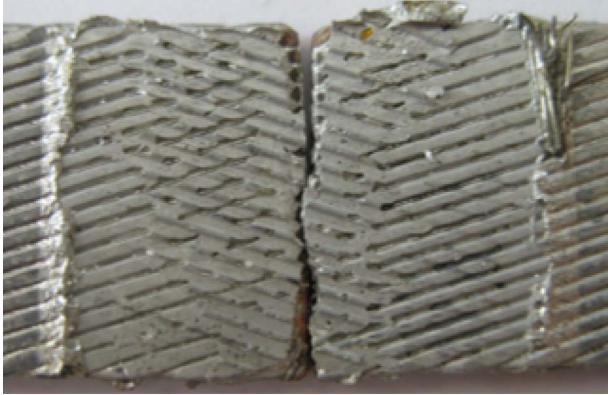
Fig. 3. Both intercable contact areas after fracturing of an LHC busbar cable splice with 10 mm cable overlap length.
