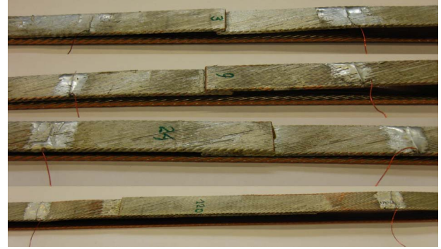
Fig. 5. Cable splices with 3, 9, 24, and 120 mm intercable contact lengths instrumented with voltage taps.
