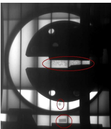
Figure 12: Radioscopy of the Diode Enclosure from the Full-size Mock-up with Particle Debris (markings)
