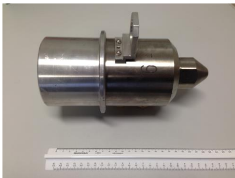
Figure 4: The figure shows the external container of a spare Antiproton Decelerator production target. The outer shell is made by Ti-6Al-4V alloy, while the inner core is composed by graphite with an iridium core.
