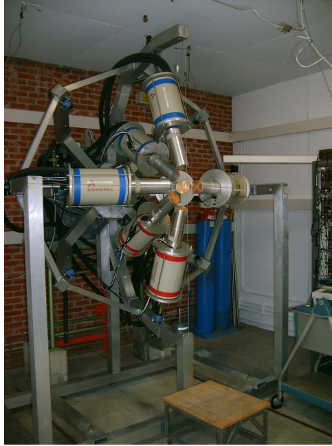
Fig. 1: The GAINS array used at EC-JRC-IRMM to determine the neutron inelastic cross sections on ^{28}\text{Si} .
