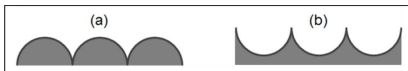
Fig. 15: Two examples of surface morphology with the same roughness parameters, but very different behaviour with respect to the EM field.
