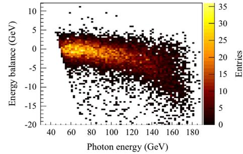
Fig. 85. Difference between the beam energy and the total measured energy as a function of the photon energy.
