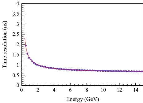
Fig. 49. Standard deviation  $\sigma$  for the ECAL2 time resolution as a function of the photon energy  $E$ . The solid curve is a fit to the data points using the expression:  $\sigma^2(E) = 1.13/E + 0.22/E^2 + 0.39$ .
