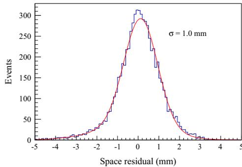
**Fig. 37.** Rich Wall residual distribution, showing the difference between reconstructed cluster position and extrapolated track position along the axis perpendicular to the wire layer. The quoted sigma is extracted by fitting a sum of two Gaussians.
