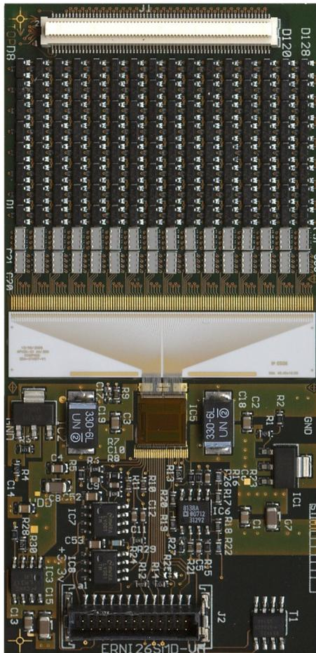
**Fig. 26.** Front-end card carrying (from top to bottom) the 130-pin connector, the protection network, a ceramic pitch adaptor, and the APV25-S1 ASIC for analog sampling of the signals induced on the readout electrodes.
