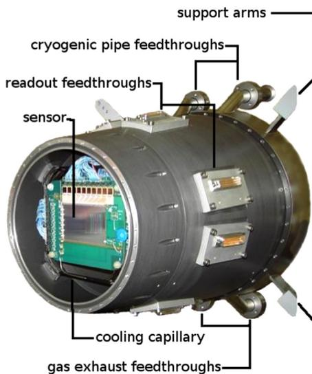
**Fig. 17.** The conical cryostat with the upstream beam window dismounted. The height of the PCB frame that holds the detector (sensor) is about 100 mm, the length of the full cryostat about 400 mm. The bent cooling capillary is fixed to the PCB close to the sensitive area of the detector. Inside the cryostat, the readout cables are directly soldered to the detector module and plugged to vacuum-sealed feedthrough connectors also visible on the outer surface of the cryostat.
