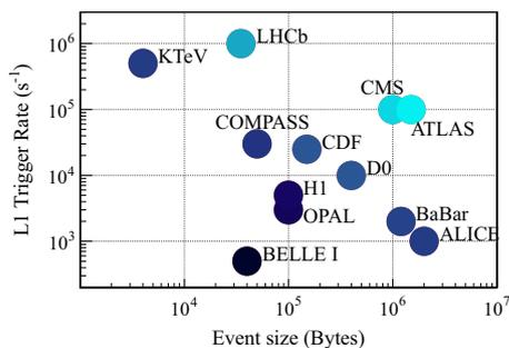
**Fig. 60.** Trigger rate versus event size. The COMPASS DAQ system is compared to several large-scale experiments. The comparison is done for first-level (L1) triggers or their equivalent.
