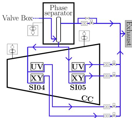
**Fig. 19.** Block diagram of the conical cryostat (CC), symbols as in Fig. 18. The phase separator is mounted in an extra housing outside the spectrometer acceptance with a vacuum connection to the cryostat.
