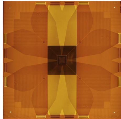
**Fig. 24.** The PixelGEM read-out foil. The inner  $10 \times 10 \text{ cm}^2$  darkest part is the active area. The symmetric wires connecting the pads and the strips to the read-out electronics surround this part.
