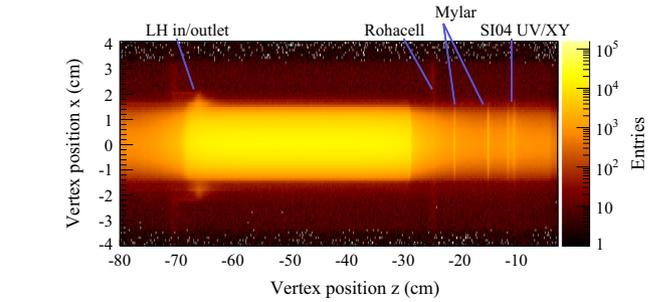
**Fig. 70.** Vertex distributions for the liquid hydrogen target ( $xz$  projection) for events with three charged tracks. For the explanation of the structures, see also Fig. 12.
