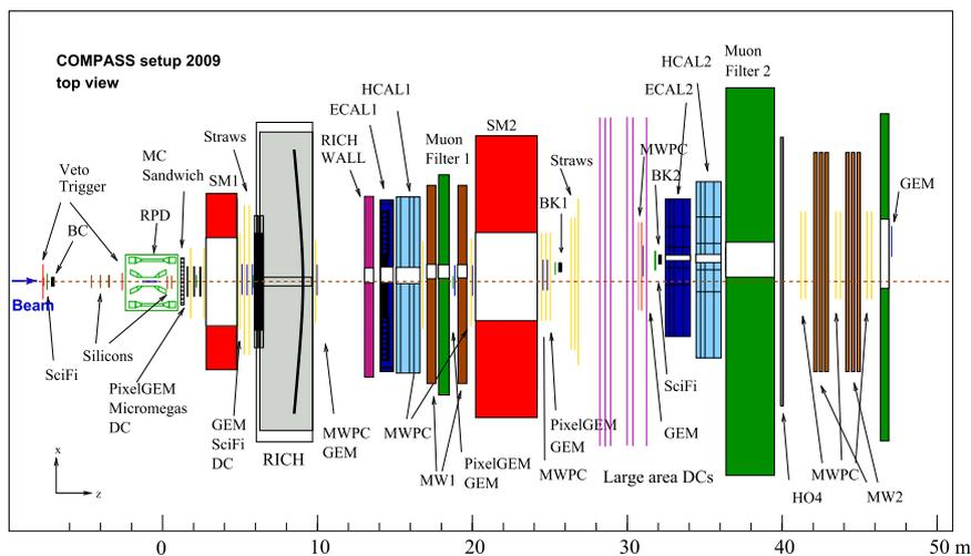
**Fig. 3.** Top view of the COMPASS setup for data taking with hadron beams. The labels indicate the various detectors, as referenced throughout this paper. The vertical scale is only indicative of the relative detector sizes. The colour code follows that of Fig. 2. (For interpretation of the references to color in this figure caption, the reader is referred to the web version of this paper.)
