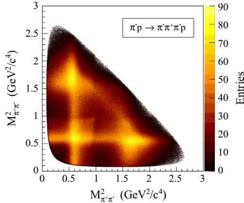
**Fig. 101.** Dalitz plot for three diffractively produced charged pions after a cut of  $\pm 130 \text{ MeV}/c^2$  around the  $\pi_2(1670)$  mass.
