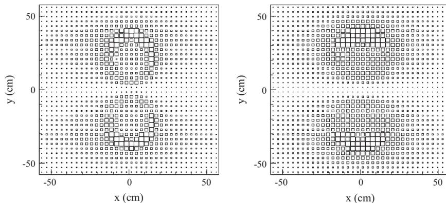
**Fig. 40.** Two-dimensional hit distributions in the central part of the RICH-1 photon detectors for (left) data taken with a muon beam and (right) data taken with a positive hadron beam.
