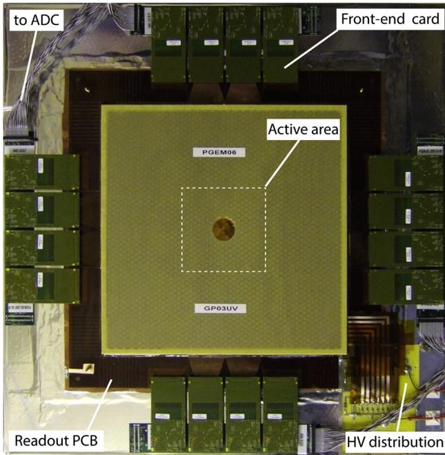
**Fig. 25.** A fully assembled PixelGEM detector, equipped with 16 APV front-end cards. The digitisation of the analog signals from the APVs is done at an external ADC card, which is connected via the grey cables.
