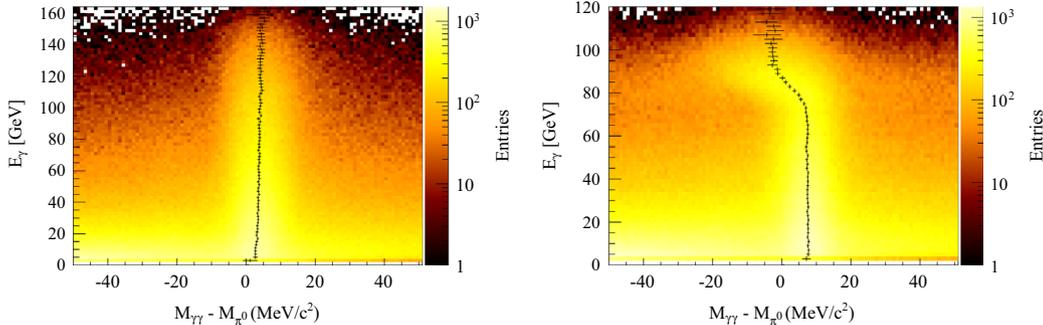
**Fig. 81.** Energy deposition in two ECAL2 modules as a function of the difference between reconstructed and nominal  $\pi^0$  mass for (left) a module with typical behaviour and (right) a module with an unusual behaviour.
