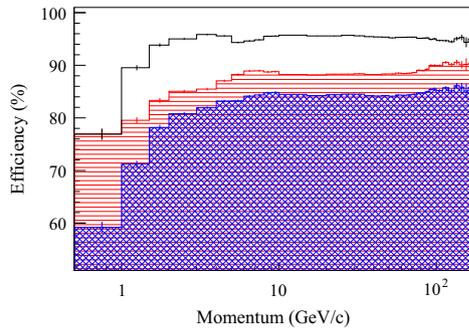
**Fig. 64.** Efficiency of tracking and vertexing as a function of momentum with the efficiency of tracking software (solid line), setup efficiency (hatched area), and overall efficiency (crossed area).
