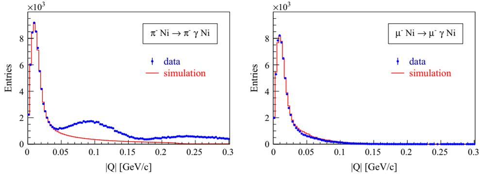
Fig. 97. Momentum transfer distributions for exclusive (left)  $\pi^- \gamma$  and (right)  $\mu^- \gamma$  events. The data (dotted lines) are compared to the MC simulation (solid lines).
