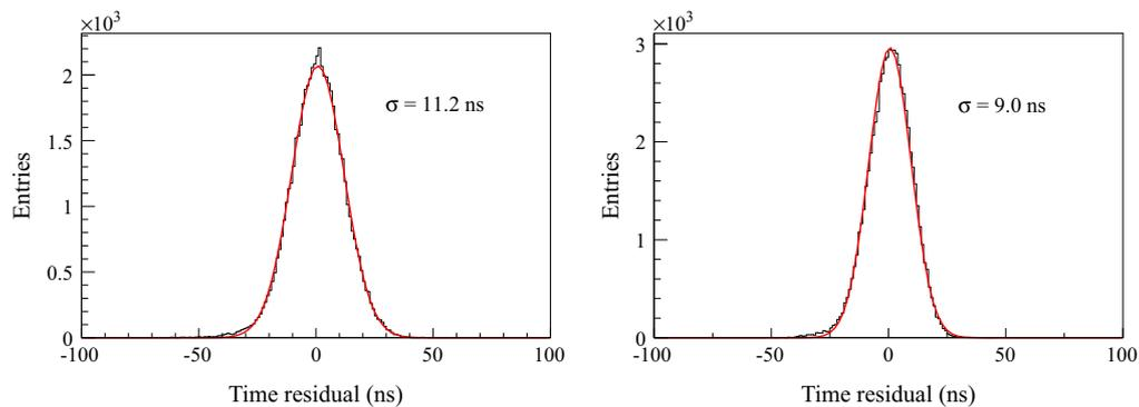
**Fig. 28.** Time residual distribution (difference between measured cluster time and track time) for (left) the pixel region and (right) the strip region ( $x$ -direction) of a PixelGEM detector.
