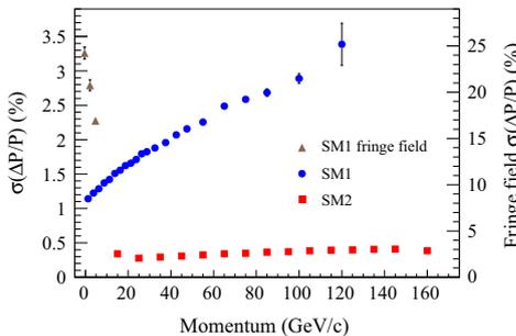
**Fig. 65.** Relative momentum resolution as a function of track momentum. The standard deviation of the reconstruction error is shown for tracks deflected by the SM2 magnet alone or by both SM1 and SM2 (squares), by the SM1 magnet alone (circles) and for those deflected by the fringe field of SM1 only (triangles, right scale).
