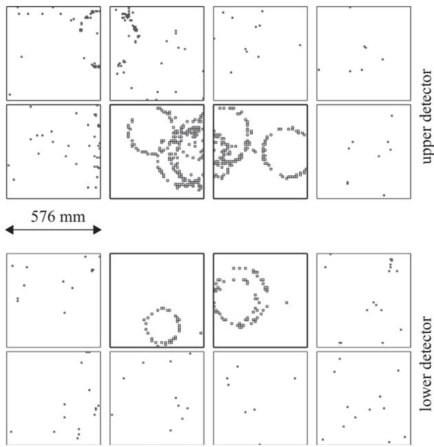
**Fig. 39.** A typical event display during hadron data taking. The 16 squares represent the detector areas; the four central ones are equipped with MAPMTs. The small squares represent the hits detected in the photon detectors.
