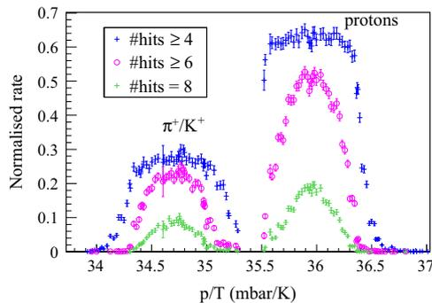
Fig. 8. Pressure scan with CEDAR1 for a positive hadron beam with at least 4, 6 or 8 PMTs in coincidence. The kaon peak cannot be distinguished from the pion peak.
