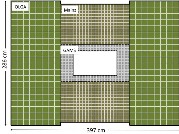
**Fig. 43.** Configuration of ECAL1. The central area is equipped with GAMS modules. The MAINZ modules are installed above and below the GAMS area. The OLGA modules cover the outer left and right regions.
