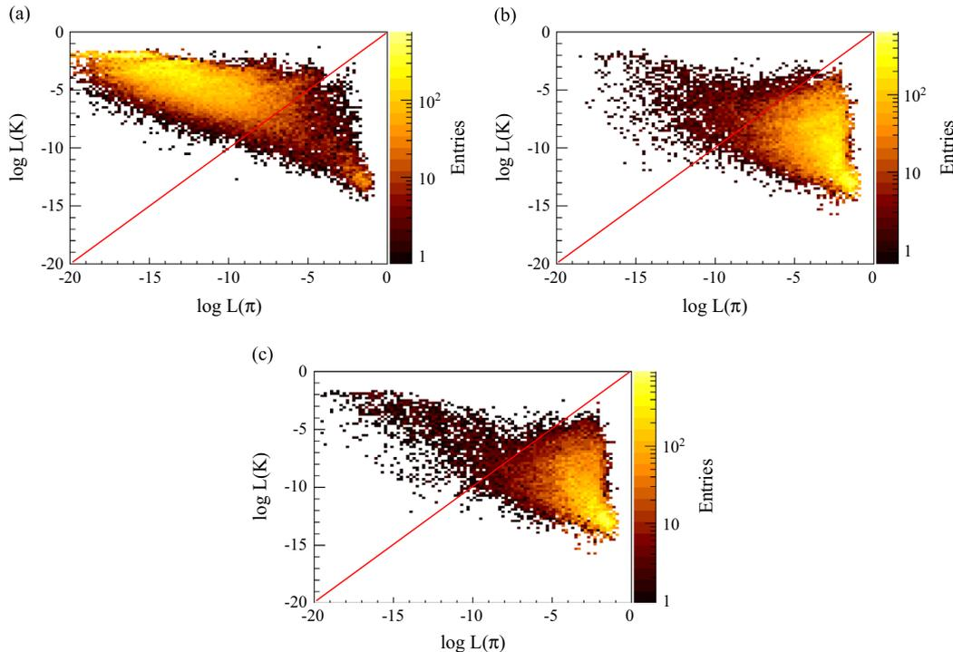
**Fig. 78.** Values for the log-likelihoods function for different samples obtained from CEDAR 2 calculated for (a) the kaon sample, (b) the pion sample and (c) an unbiased beam sample. The line indicates  $\log L(\pi) = \log L(K)$ . (a) kaon sample, (b) pion sample, and (c) beam sample.
