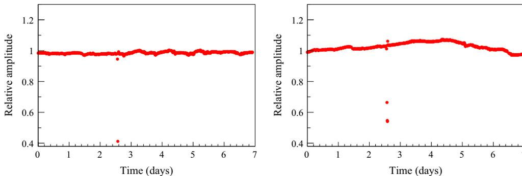
Fig. 50. ECAL2 module responses as monitored during a period of 1 week for (left) a stable module and (right) an unstable module. The vertical scale is normalised to the SADC charge measured in the beginning of the period.
