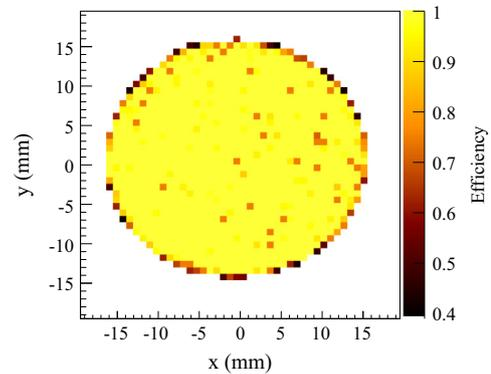
Fig. 52. Beam counter efficiency distribution in transverse coordinates.
