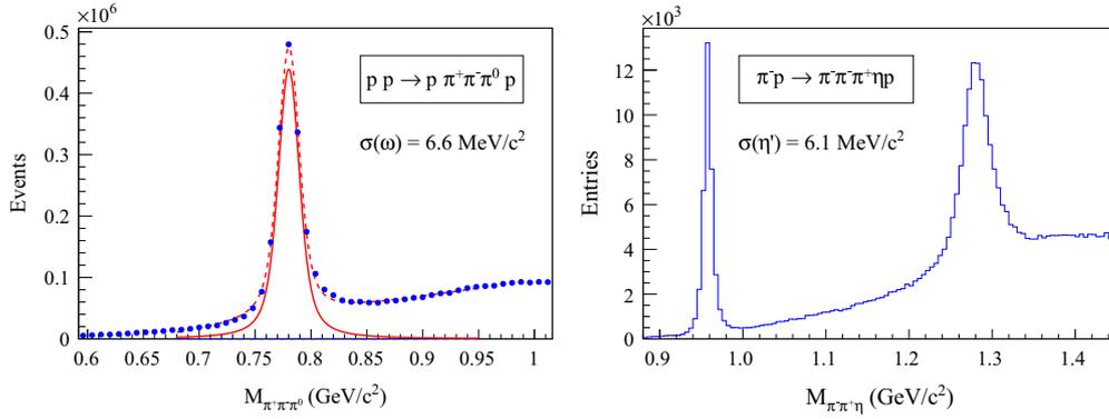
**Fig. 100.** Invariant mass spectra for (left)  $\pi^- \pi^+ \pi^0$  and (right)  $\pi^- \pi^+ \eta$  systems. The full line in the left panel is a fit to the  $\omega$  peak only; the dashed line includes also the background.
