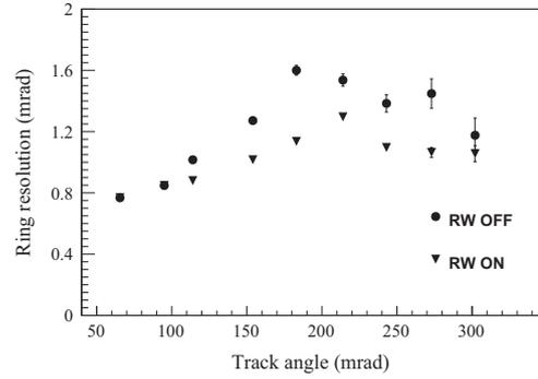
**Fig. 38.** Resolution of the reconstructed Cherenkov ring for pions as a function of the track angle. The two different trends in the curve below and above  $\sim 175$  mrad are due to the different RICH-1 photon detector types (see Section 6.1).
