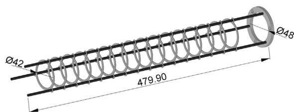
Fig. 13. Schematic view of the target holder used for measurements with nuclear targets.
