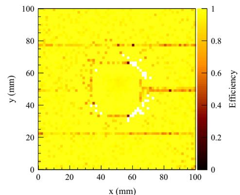
**Fig. 29.** Efficiency of one of the PixelGEM detectors, measured in a high-intensity hadron beam. The horizontal lines with reduced efficiency correspond to boundaries between GEM sectors. In the white region not enough tracks are reconstructed when this particular detector is excluded from the tracking.
