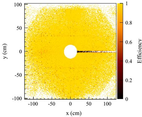
Fig. 32. Two-dimensional representation of the efficiency for one of DC4 layers. The half horizontal lines with reduced efficiency indicate the position of the power supply lines of the beam killer.
