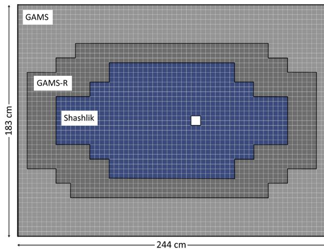
**Fig. 46.** Configuration of ECAL2. The outer and intermediate regions are equipped with GAMS and radiation-hardened GAMS modules respectively. The inner region is equipped with Shashlik sampling modules. The transverse sizes of all three types of modules are identical. The central hole of  $2 \times 2$  modules can be seen as a white spot.
