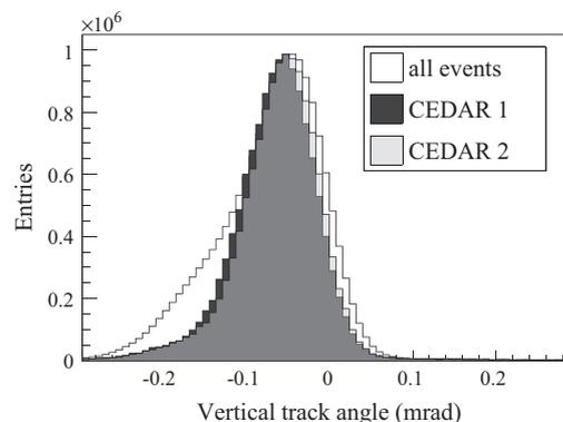
Fig. 10. Horizontal (left) and vertical (right) track angles at the CEDARs. The angles for all tracks measured by the silicon beam telescope and propagated back to the CEDAR positions are compared to the angles of the tracks accepted by CEDAR1 or CEDAR2. The acceptance of the CEDARs is reduced significantly for very divergent beam tracks.
