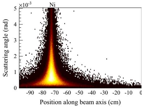
Fig. 89. Monte Carlo simulation of the Primakoff-Compton reaction, showing the reconstructed position of the primary vertex along the beam direction as a function of the scattering angle of the outgoing pion. Note that interactions outside the target material are not simulated.
