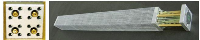
**Fig. 47.** Photographs of a Shashlik-type calorimeter module. *Left part:* the upstream face of the module with its four central rods and 16 light fibres. *Right part:* the module itself with the fibres guide at the downstream face.
