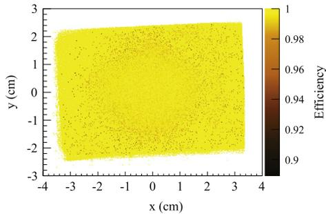
**Fig. 22.** Two-dimensional efficiency distribution for a plane in the beam telescope. The stereo-angle tilt of the sensitive area is visible.
