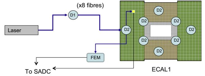
**Fig. 44.** Schematic view of the LASER monitoring system for ECAL1. The laser beam is distributed to the ECAL1 modules using one primary (D1) and eight secondary (D2) light diffusion spheres. For clarity, only one of the eight primary fibres dispatching the light to D2, only one of the secondary 1500 fibres transmitting it to the LG modules, and only one of the eight front-end-monitoring (FEM) modules are explicitly shown.
