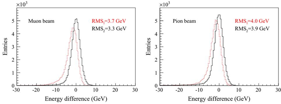
**Fig. 87.** Difference between beam and measured energies (energy balance) for Primakoff–Compton scattering (left) with a muon beam and (right) with a pion beam. The distributions are displayed with the standard  $\pi^0$  calibration only (dashed curve) and with linearity and intra-cell position corrections (solid curve); the corresponding  $\text{RMS}_1$  and  $\text{RMS}_2$  values are indicated.
