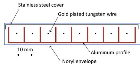
Fig. 34. Sketch of a Mini Drift Tube module.
