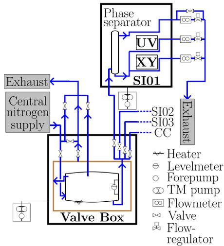
**Fig. 18.** Block diagram of the valve box and the first upstream cryostat labelled SI01. The other two upstream cryostats SI02 and SI03 are equipped analogously. The downstream conical cryostat (CC) is shown in Fig. 19. The phase separators are integrated in the cryostats near the detectors, but outside the acceptance.
