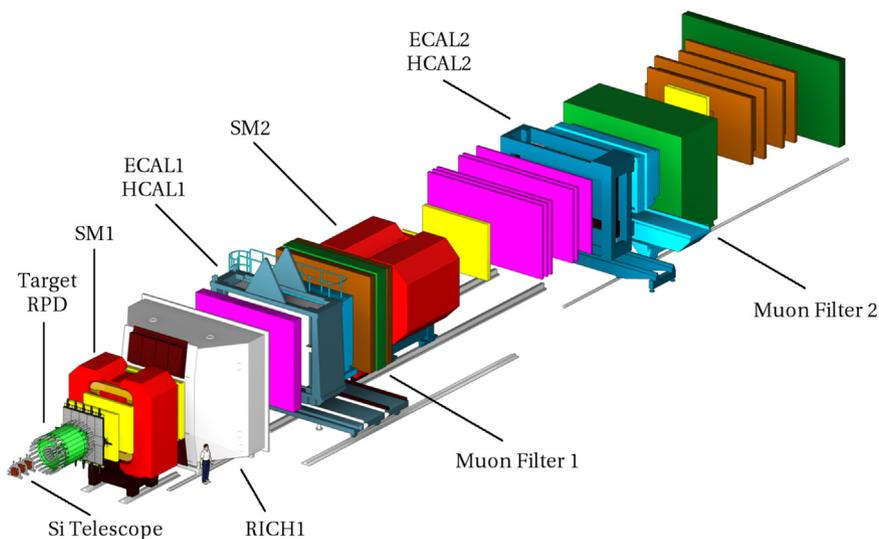
**Fig. 2.** Three-dimensional view of the COMPASS setup for measurements with hadron beams. The beam comes from the left side. The upstream part of the setup (beam line) is not shown here. The different colours indicate different detector types. (For interpretation of the references to color in this figure caption, the reader is referred to the web version of this paper.)
