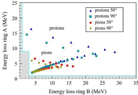
**Fig. 55.** Correlation between the energy losses of protons and pions traversing ring A and stopping (or traversing) ring B of the RPD. For each particle type the minimum and the maximum polar angles ( $50^\circ$  and  $90^\circ$ ) are shown. The shaded area corresponds to the region rejected by the trigger logic.
