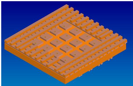
**Fig. 23.** Schematic view of the pixel and strip region of the readout circuit. Note that the pixel region consists of  $32 \times 32$  pixels of  $1 \text{ mm}^2$  size each, while only  $4 \times 4$  are shown for clarity. Figure not to scale.
