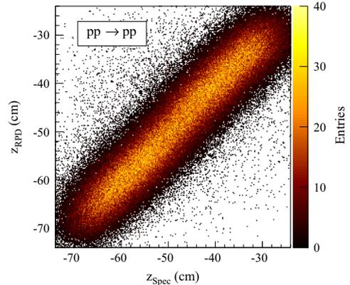
**Fig. 71.** Correlation between the longitudinal vertex position  $z$  determined with the RPD and the one determined with the spectrometer.
