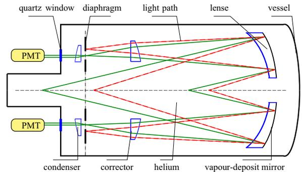
**Fig. 6.** The basic principle of a CEDAR counter. Two particles with the same momentum but with different masses (here full and dashed lines) radiate Cherenkov photons at different angles, resulting in rings with different radii. A diaphragm selects the rings from the required particle type.
