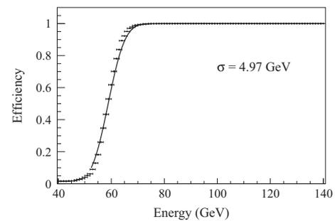
Fig. 58. Efficiency of the ECAL2 trigger as a function of the energy. The solid line is a fit to the data with an error function.
