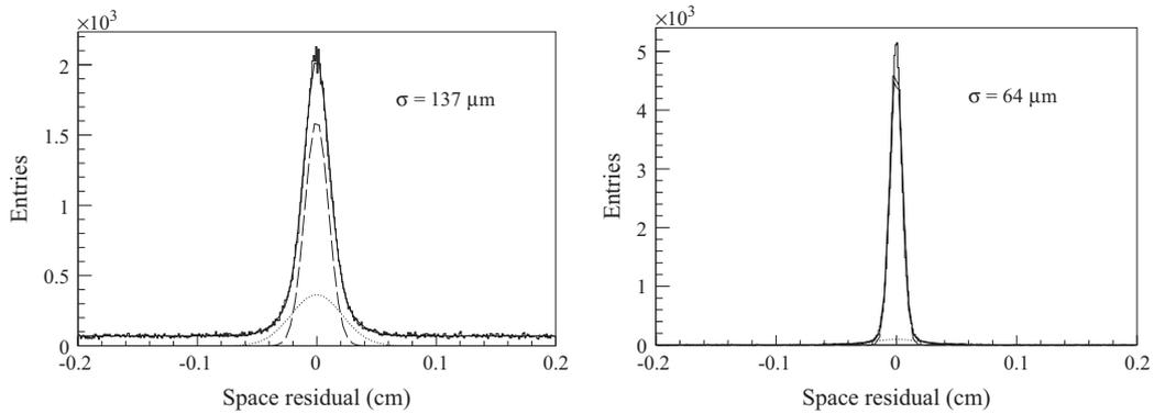
**Fig. 27.** Residual distribution (difference between measured cluster position and track penetration point) in  $x$ -direction for (left) the pixel region and (right) the strip region of a PixelGEM detector. The quoted residual widths are obtained from fits of a sum of two Gaussians. When corrected for the track uncertainties, spatial resolutions of  $106 \mu\text{m}$  (pixels) and  $54 \mu\text{m}$  (strips) are obtained for this particular detector.
