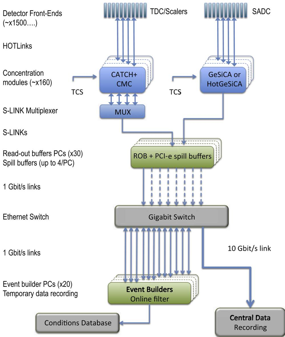
**Fig. 61.** Overview of the COMPASS DAQ system. Data coming from the detectors are first digitised in the front-end cards and then merged in the concentrator modules, either CATCH or GeSiCA(HotGeSiCA). The data from the concentrator modules are first sent to the readout buffers and then transmitted to the event builders. The data are temporarily saved on disk, before being migrated to the central data recording facility.
