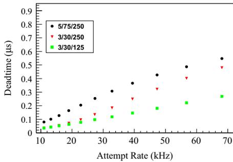
Fig. 62. Data acquisition dead time for three different TCS settings, as measured as a function of the attempted trigger rate. The settings used in 2008/2009 are shown in triangles.
