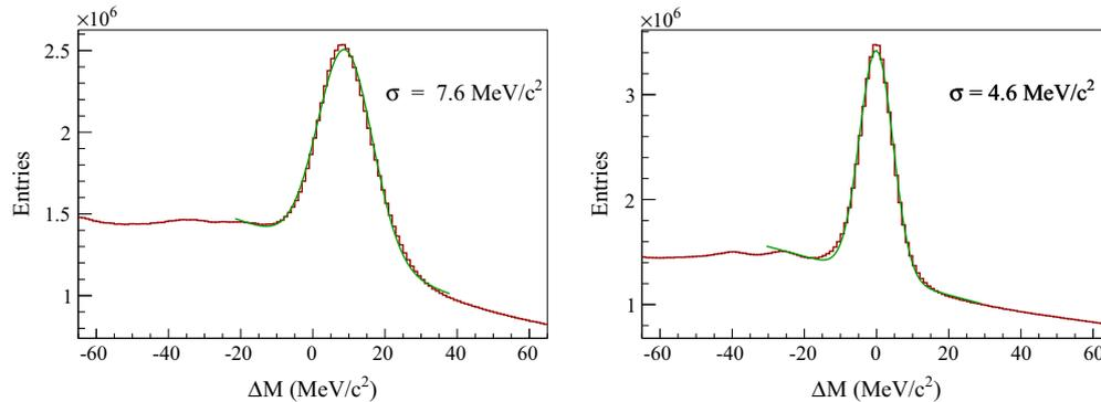
**Fig. 82.** Difference  $\Delta M$  between reconstructed and nominal  $\pi^0$  masses in ECAL2 for (left) before calibration and (right) after calibration.
