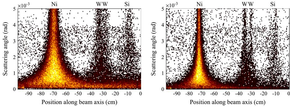
**Fig. 67.** Distribution of scattering angle of the outgoing pion vs. the position of primary vertex along the beam axis from Primakoff data, illustrating the improvement of the vertex resolution between (left) standard alignment and (right) run-by-run alignment. The structures correspond to interactions in the different targets used in the measurement (see Table 3) and in the first silicon station downstream of the targets.
