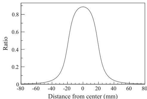
**Fig. 79.** Shower reconstruction: (left) fraction of total shower energy collected from  $-\infty$  up to a particular distance from the shower center (Eq. (8)); (right) fraction of the total energy deposited in a column as a function of its distance from the shower center.
