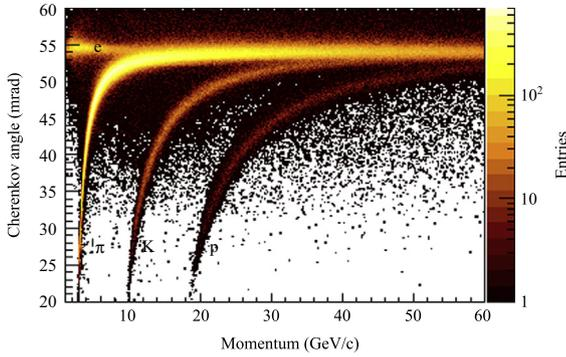
**Fig. 74.** Cherenkov angle for reconstructed rings as a function of the particle momentum for the  $C_4F_{10}$  radiator.
