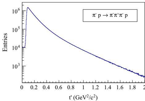
Fig. 94. Squared four-momentum transfer for  $\pi^- \pi^+ \pi^-$  events produced by a pion beam impinging on a liquid hydrogen target, and selected by the DTO trigger.
