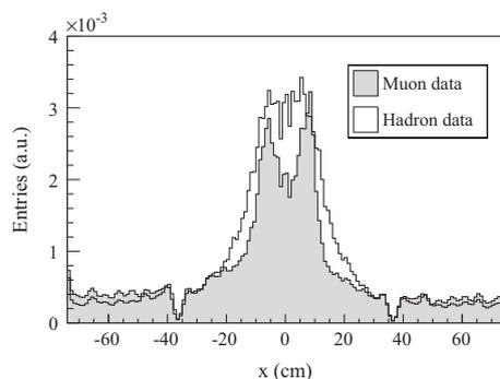
**Fig. 41.** Horizontal axis projection of the integrated hit distributions for the lower photon detectors. Both central and peripheral parts of RICH-1 are included. The shaded histogram refers to the muon environment, the open to the hadron one. The small dips in the hit distributions correspond to the dead zones between the detector parts equipped with MAPMTs and with MWPCs.
