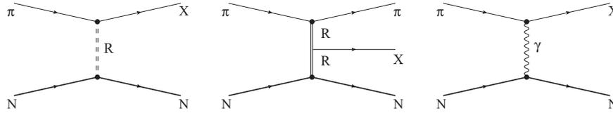
**Fig. 1.** Production mechanisms employed in COMPASS for (left) diffractive dissociation, (middle) central production, (right) photo-production by quasi-real photons  $\gamma$ , with  $\pi$  denoting the beam particle (can be also  $p, K$ ), and  $N$  is the target nucleon or nucleus.
