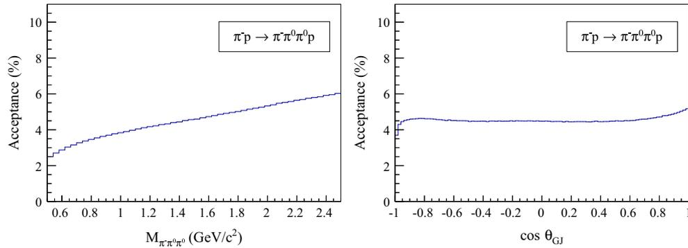
Fig. 92. Acceptance for the diffractively produced  $\pi^- \pi^0 \pi^0$  final state (left) as a function of the  $3\pi$  invariant mass and (right) as a function of the polar angle of the  $\pi^0 \pi^0$  isobar in the Gottfried–Jackson frame.
