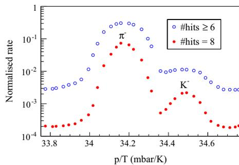
Fig. 9. Pressure scan with CEDAR1 for a negative hadron beam with at least 6, or with 8 PMTs in coincidence.
