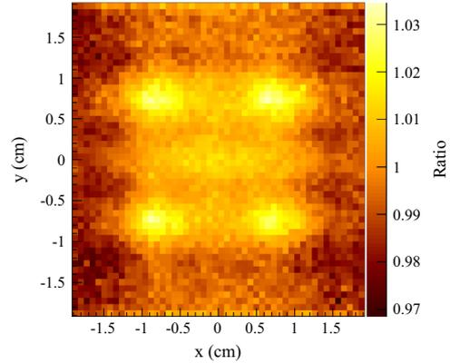
Fig. 84. Ratio of track momentum over calorimeter energy as a function of the impact position in a Shashlik module relative to its centre. The four central spots with a ratio larger than one correspond to the four module rods.
