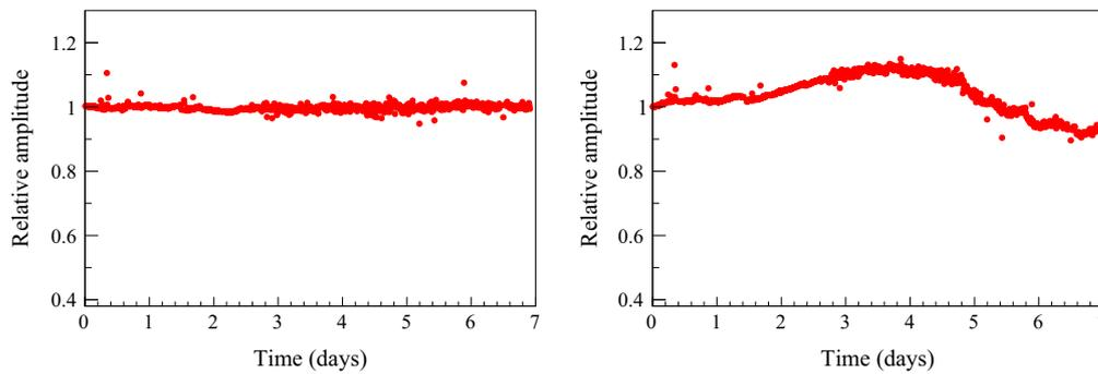
**Fig. 45.** ECAL1 module responses as monitored during a period of 1 week for (left) a stable module and (right) an unstable module. The vertical scale is normalised to the SADC charge measured in the beginning of the period.
