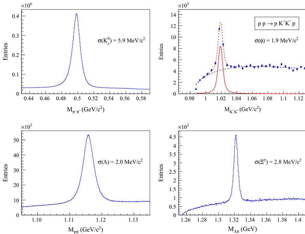
Fig. 99. Reconstructed invariant masses for charged particles in the final state. The peaks shown are for (top left)  $K_s^0(498)$ , (top right)  $\phi(1020)$ , (bottom left)  $\Lambda(1115)$ , and (bottom right)  $\Xi^\pm$ . The  $K_s^0$ ,  $\Lambda$ , and  $\Xi^\pm$  particles are produced in inclusive reactions. The dashed curve in the  $\phi(1020)$  plot is a fit to the background.
