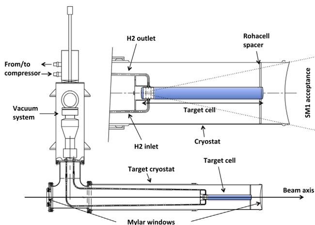
Fig. 12. Side view of the liquid hydrogen target system. A closer view of the cylindrical Mylar cell and hydrogen piping is shown in the inset.
