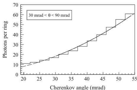
**Fig. 42.** Mean number of detected photons per reconstructed ring as a function of the corresponding Cherenkov angle  $\theta_{ch}$  in the central region of the RICH-1 detector for track angles  $\theta$  between 30 mrad and 90 mrad. The line is a fit with the functional form  $N = N_0 \sin^2(\theta_{ch})$ .
