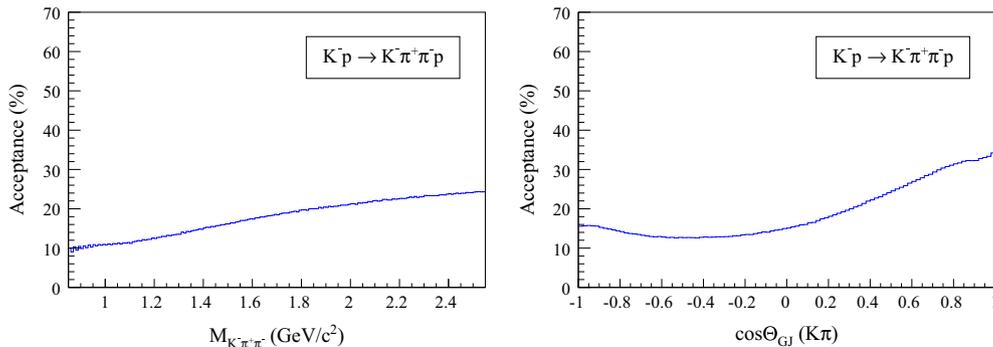
Fig. 91. Acceptance for the diffractively produced  $K^-\pi^+\pi^-$  final state (left) as a function of the  $K\pi\pi$  invariant mass, and (right) as a function of the polar angle of the  $\pi^+K^-$  isobar in the Gottfried-Jackson frame.
