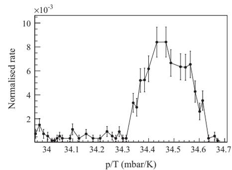
Fig. 11. Count rate of coincident events recorded with CEDAR1 and CEDAR2. The pressure of CEDAR2 was scanned while CEDAR1 was set to detect kaons.
