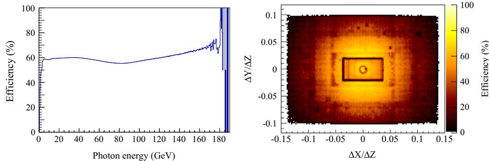
**Fig. 88.** Simulated photon efficiency (left) as a function of the photon energy and (right) as a function of the photon direction in the laboratory system.
