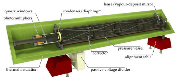
**Fig. 7.** A cut through one of the CEDAR detectors.
