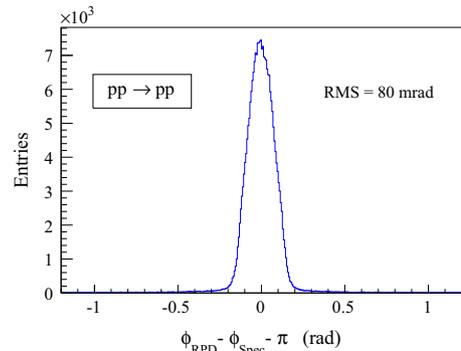
**Fig. 72.** Correlation between the azimuthal angles of the recoil proton detected in the RPD and the scattered proton detected in the spectrometer.
