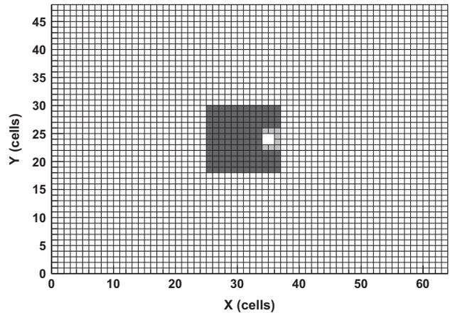
Fig. 57. The active area of the ECAL2 trigger (shown in dark grey). The cells shown in light grey are rejected due to high rates.
