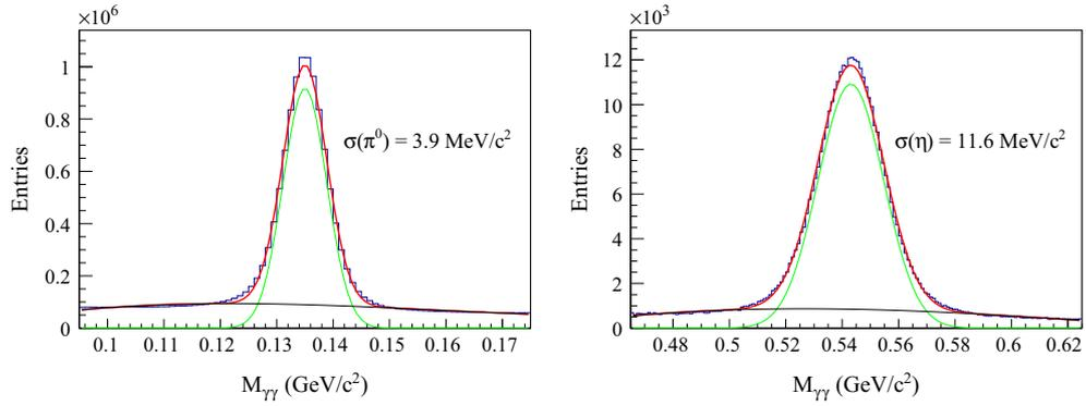
Fig. 98. Two-photon invariant mass distribution as measured in ECAL2, in the (left)  $\pi^0$  mass region and (right)  $\eta$  mass region. The solid curves are fits to the signal and to the background. The values of the resolution achieved are indicated in each plot.
