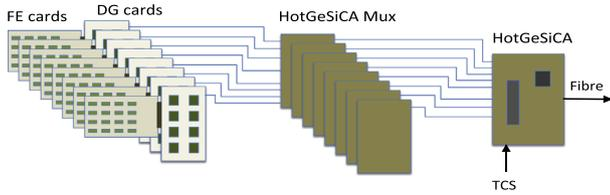
**Fig. 36.** Schematic view of the Rich Wall readout chain.
